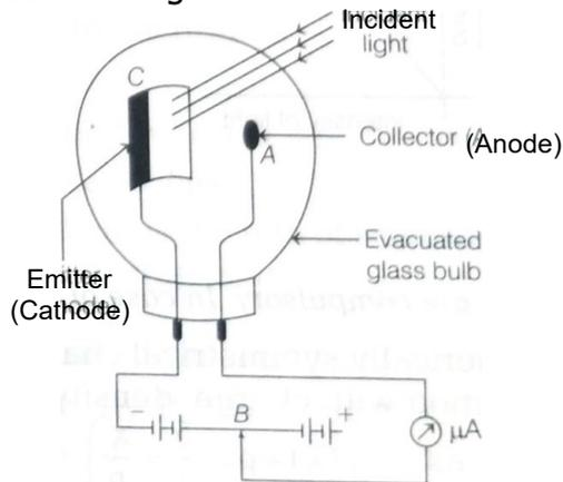
A photocell consists of a semi-cylindrical photosensitive metal plate C (emitter) and a wire loop A (collector) supported in an evacuated glass or quartz bulb. When light of suitable wavelength falls on the emitter C, photoelectrons are emitted.
